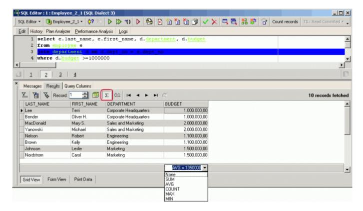
Then select the aggregate function from the drop-down list for each NUMERIC / DATETIME column as required.
