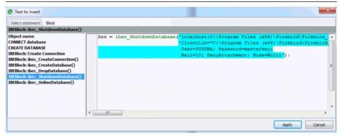
By dragging a table or view name, all fields are automatically inserted in to the editor. Single or multiple fields can be dragged from a single table, by selecting with the [Ctrl] or [Shift] key depressed. Here the following statements are offered:
