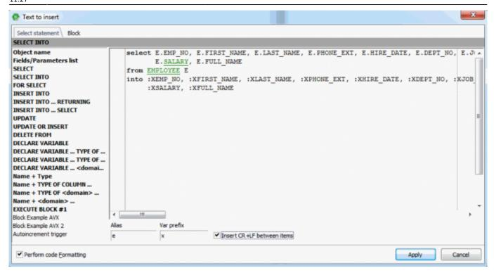
Here you can also quickly create your table aliases by entering a table alias just once, it is then automatically inserted after the table name and as a prefix for all relevant fields. And check the *CR+LF* (Carriage Return/Linefeed) box if you'd like your code to be aligned.
