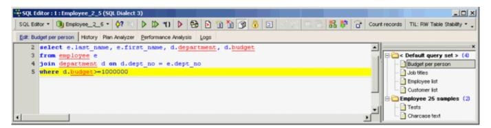
Firebird 2.0 blocks can also be debugged directly in the SQL Editor (or alternatively in the Block Editor) using the Block Debugger. Simply click the *Debug* icon to open the Block Editor:
