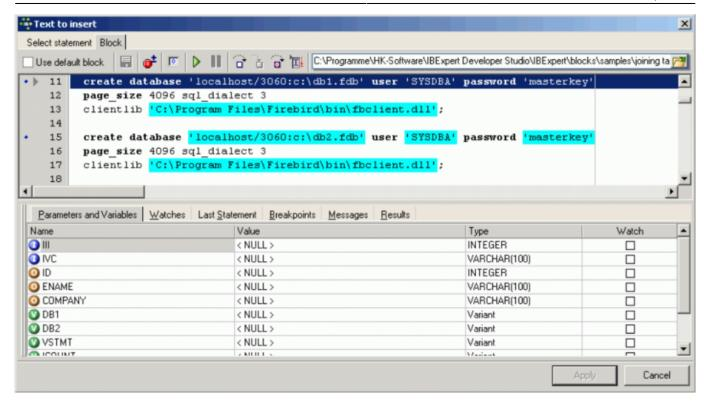
You can use the Default Block (checkbox option), one of the IBEBlock samples or load your own customized IBEBlock (for example, Default Block adapted to include domains. Further information can be found in the IBEBlock documentation.
