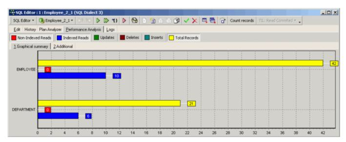
The x-axis lists the names of the tables consulted by the query/procedure, with the number of operations displayed graphically. Click the performance type you wish to view, and it will be added to the graph. Click the button again, to remove it.
