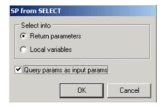
When creating a procedure from a select it is necessary to specify whether to select into return parameters or local variables.
